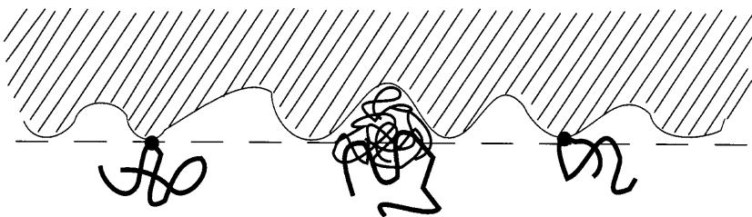
Fig. 6. A rough surface of die wall, where the stagnant ( thin ) chains allow the unbound chains (the middle thick chain without dot ) to entangle and “adsorb” at the effective interface ( dashed line ). Adsorbed chains ( thick chains with dots ) are also present. Such an interface can also produce a stick-slip transition upon a coil-stretch transition involving the thick chains. See Ref. [27]. For clarity, we only draw three “tethered” chains (two adsorbed and one entangled) besides the stagnant chains in one valley. The chains not drawn here, of course, fill up all the space away from the rough wall
